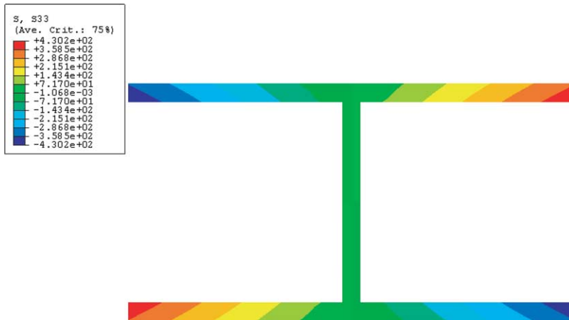
Fig. 11. \sigma_{11} for isotropic I-beam at the midspan of the beam from ABAQUS (3-D).
