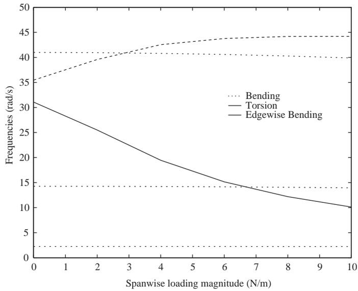
Fig. 4. The effect of geometrical nonlinearities on the structural frequencies.
