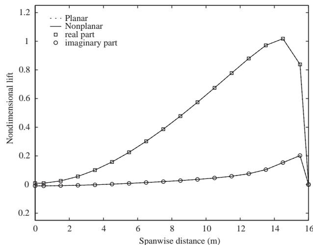
Fig. 3. The effect of geometrical nonlinearities on the lift generated by a curved wing vibrating in its first flatwise bending mode at a reduced frequency of 0.4.
