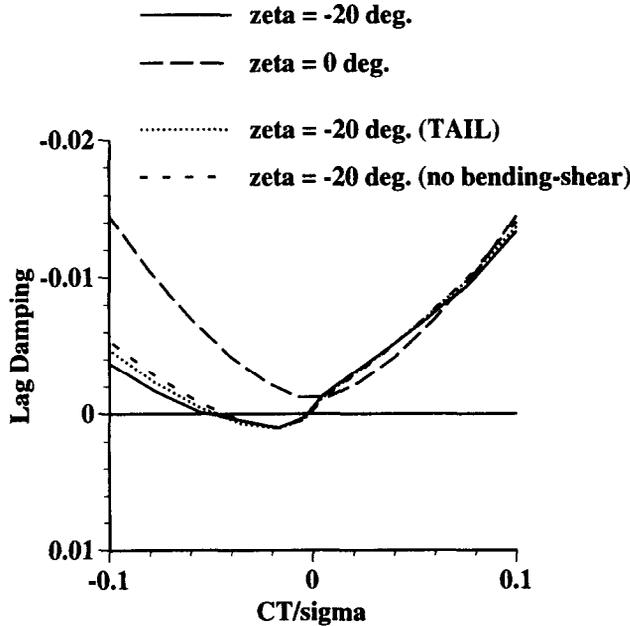
Figure 15. Normalized lag damping for  $[0_2/\zeta_4]$  box beam (L2e) for rotor R1 with various values of  $\zeta$ .
