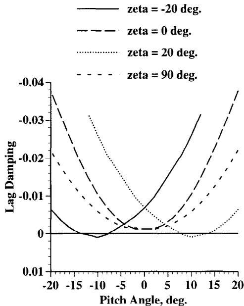
Figure 12. Normalized lag damping for  $[0_2/\zeta_4]$  box beam (L2e) for rotor R1 with various values of  $\zeta$ .
