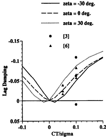
Figure 5. Lag damping for box HC I (pitch-lag coupling).
