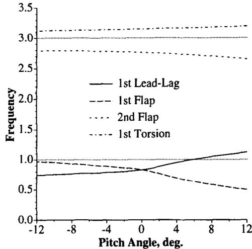
Figure 10. Normalized frequencies for rotor R2.
