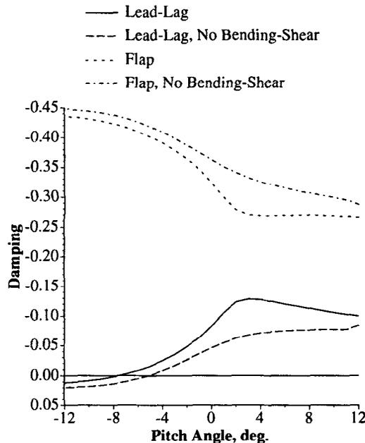
Figure 11. Normalized damping for rotor R2, with and without bending-shear coupling.
