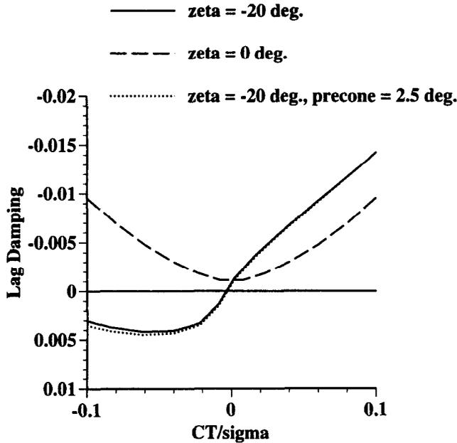
Figure 16. Variation in lag damping with the addition of 2.5° of precone for configuration R1 L3e ( $[\zeta, \zeta - 90, \zeta, (\zeta - 90)_2, \zeta]$ ).
