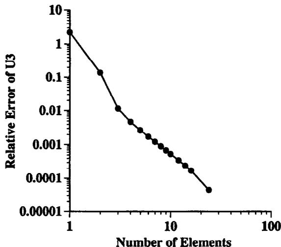
Figure 1. Absolute value of the relative error of the equilibrium value of  $u_3$  (flapwise deflection) at the tip versus number of elements for R1 L3e ( $([\zeta, \zeta - 90, \zeta, (\zeta - 90)_2, \zeta])$  with  $\zeta = 0^\circ$  and a root pitch angle of  $12^\circ$ .
