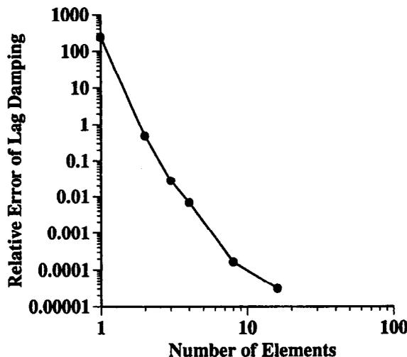
Figure 2. Absolute value of the relative error of the lead-lag damping versus number of elements for R1 L3e ( $([\zeta, \zeta - 90, \zeta, (\zeta - 90)_2, \zeta])$  with  $\zeta = 0^\circ$  and a root pitch angle of  $1^\circ$ .
