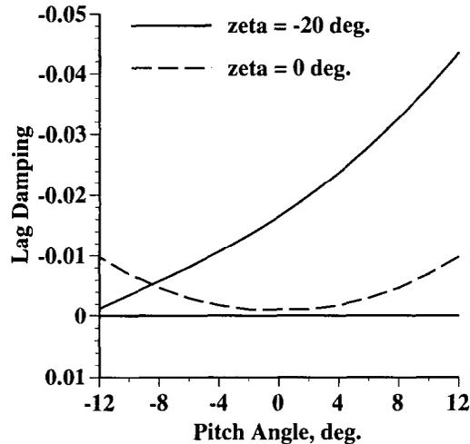
Figure 13. Normalized lag damping for  $[\zeta, \zeta - 90, \zeta, (\zeta - 90)_2, \zeta]$  box beam (L3e) for rotor R1 with two values of  $\zeta$ .
