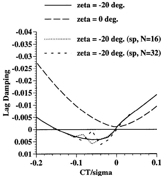
Figure 9. Plot of the eigenproblem solution’s sensitivity to machine precision for a certain range of operating conditions for R1 L3e.
