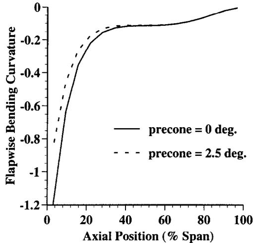
Figure 18. Plot of  $\kappa_2$  (flapwise bending curvature) for two different values of precone for  $C_T/\sigma = 0.21$  for R1 L3e ( $(\zeta, \zeta - 90, \zeta, (\zeta - 90)_2, \zeta)$ ) with  $\zeta = -20^\circ$ .
