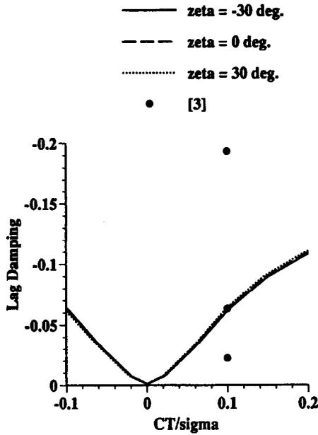
Figure 7. Lag damping for box HC III (extension-twist coupling).
