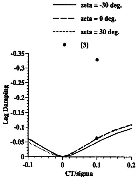
Figure 8. Lag damping for box HC IV (extension-twist coupling).
