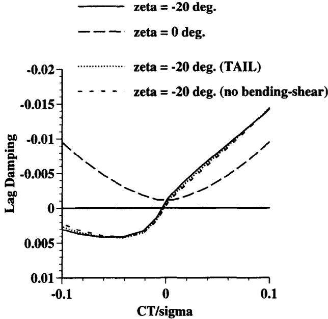
Figure 14. Normalized lag damping for  $[\zeta, \zeta - 90, \zeta, (\zeta - 90)_2, \zeta]$  box beam (L3e) for rotor R1 for two values of  $\zeta$ .
