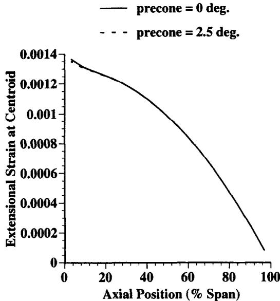
Figure 17. Plot of  $\gamma_{11}$  (extensional strain) for two different values of precone for  $C_T/\sigma = 0.21$  for R1 L3e ( $[\zeta, \zeta - 90, \zeta, (\zeta - 90)_2, \zeta]$ ) with  $\zeta = -20^\circ$ .
