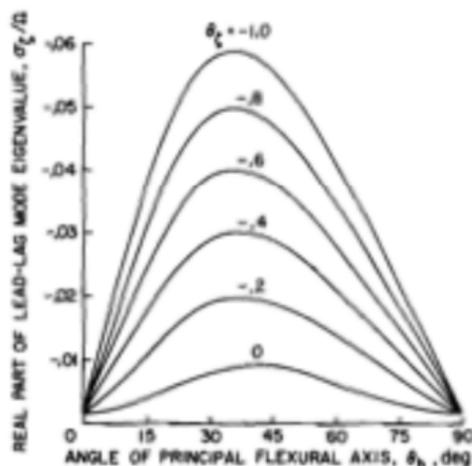
Figure 1. Effect of inclination of principal flexural axes on lead-lag mode damping at zero pitch angle ( $\theta = 0^\circ$ ),  $p = 1.1$ ,  $\omega_{c0}/\Omega = 0.7$ ,  $\gamma = 8$ ,  $2c_d/p = 0.01/\pi$ ,  $R = 1.0$ .
