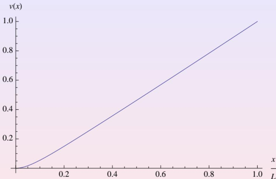
Figure: Fundamental flapping displacement mode shape of a rotating clamped-free beam with zero hub offset for  $\Omega = 25\sqrt{\frac{EI}{mL^4}}$
