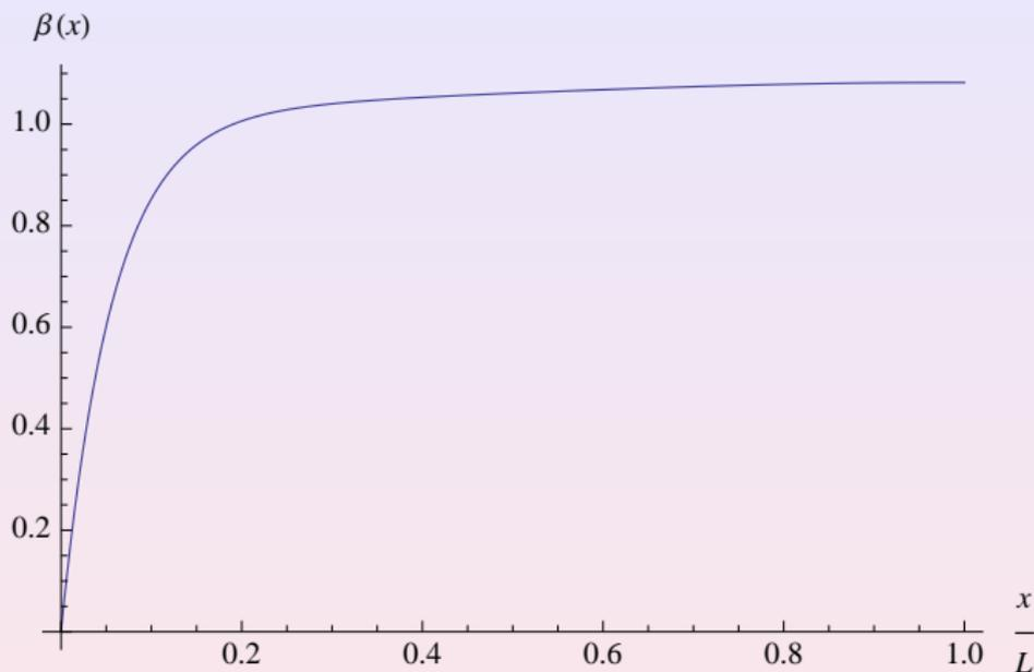
Figure: Fundamental flapping slope mode shape of a rotating clamped-free beam with zero hub offset for  $\Omega = 25\sqrt{\frac{EI}{mL^4}}$
