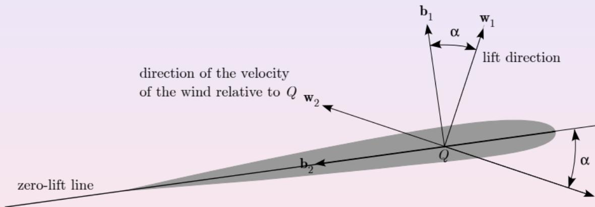
Figure: Schematic of rotor blade airfoil showing unit vectors
