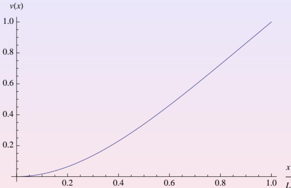
**Figure:** Fundamental flapping displacement mode shape of a nonrotating clamped-free beam with zero hub offset
