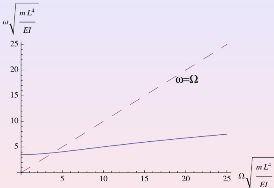
**Figure:** Fundamental natural lead-lag frequency of a rotating clamped-free beam with zero hub offset versus angular speed
