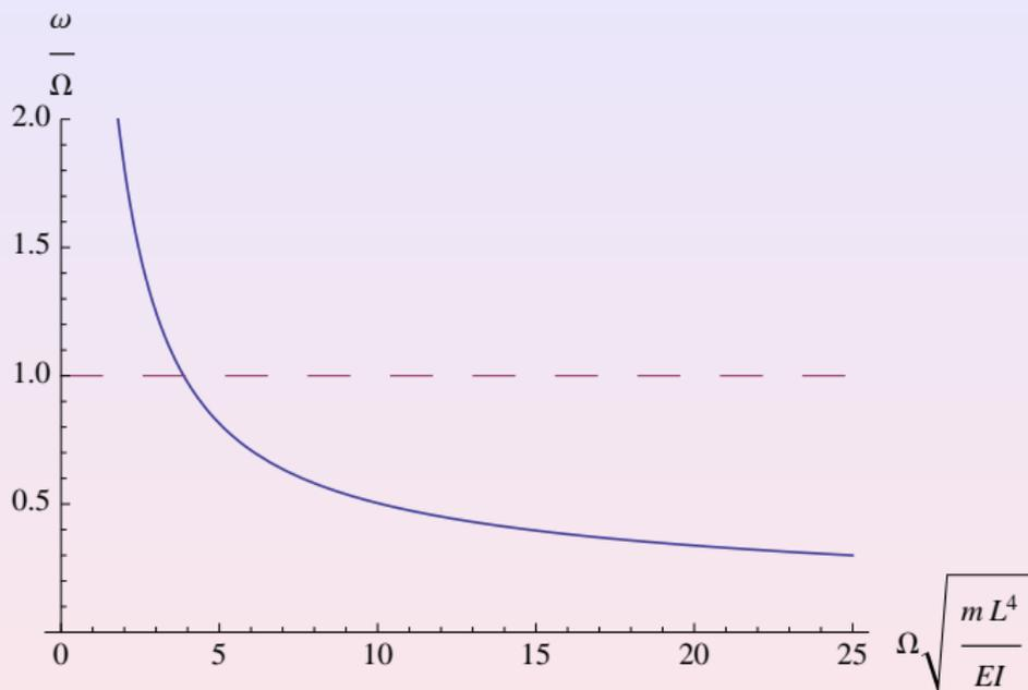
Figure: Fundamental natural flapping frequency (per rev) of a rotating clamped-free beam with zero hub offset versus angular speed
