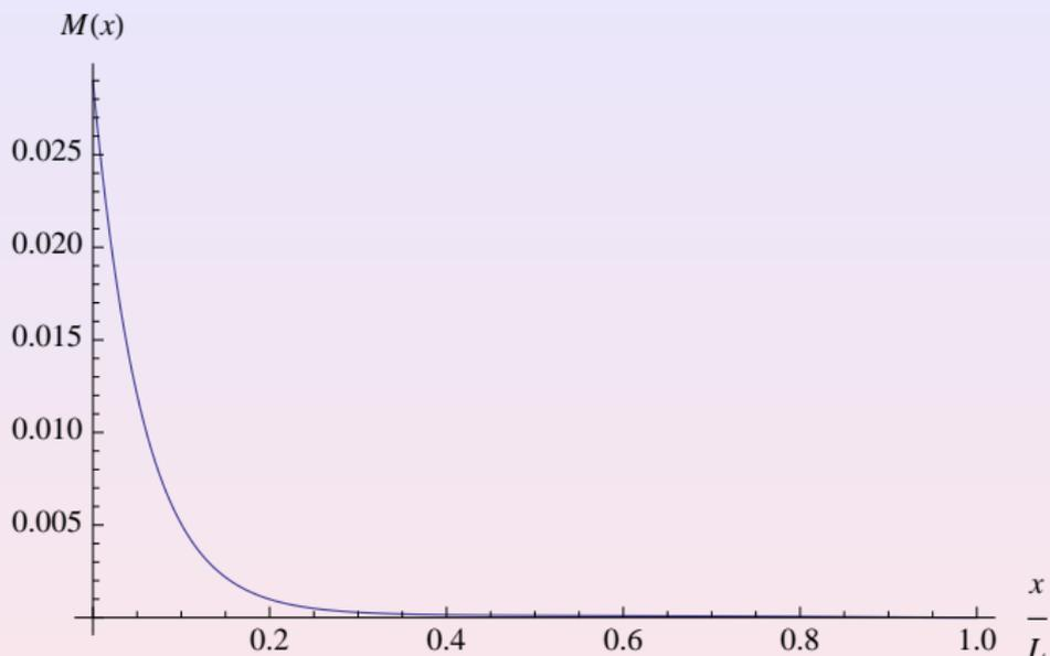
Figure: Fundamental flapping moment mode shape of a rotating clamped-free beam with zero hub offset for  $\Omega = 25\sqrt{\frac{EI}{mL^4}}$
