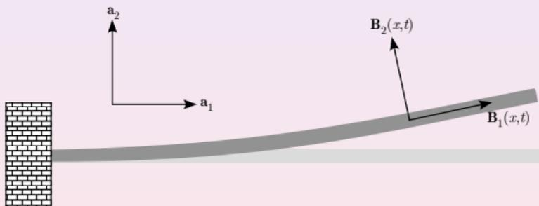
**Figure:** Schematic of cantilevered beam rotating about an axis fixed in inertial space and parallel to  $\mathbf{a}_2$
