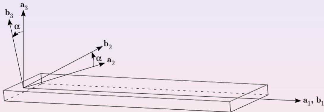
Figure: Blade-like rigid body with pitch angle  $\alpha$
