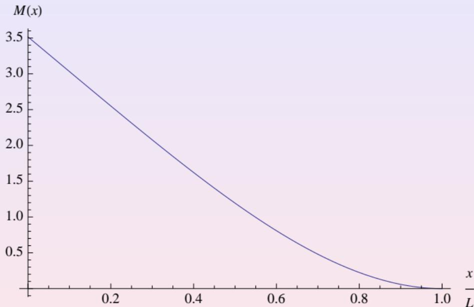
**Figure:** Fundamental flapping moment mode shape of a nonrotating clamped-free beam with zero hub offset
