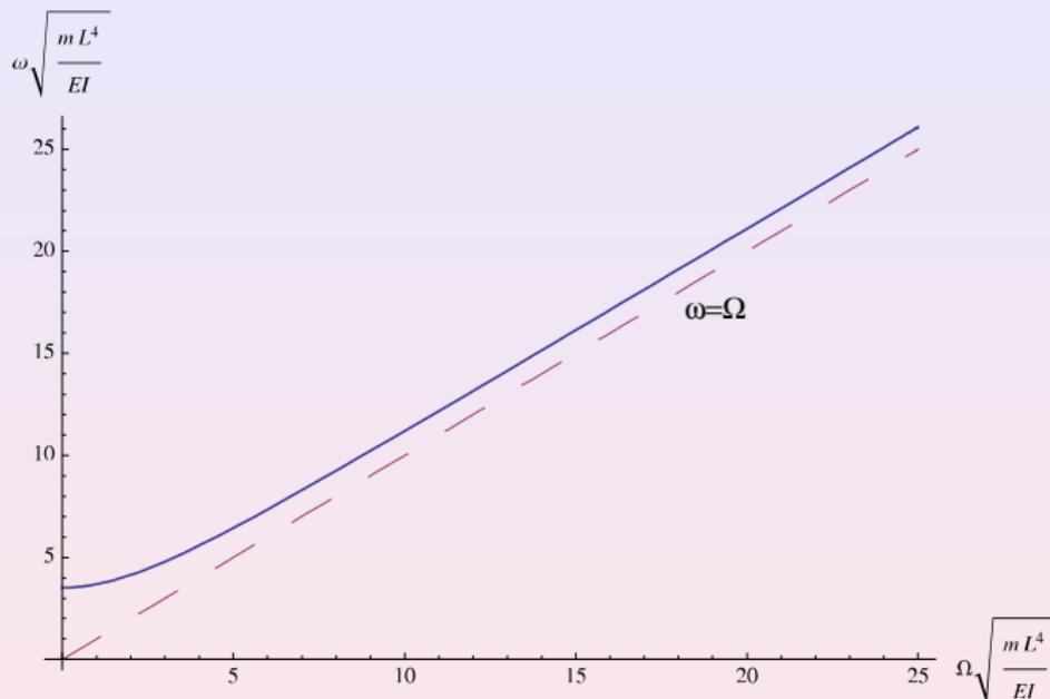
**Figure:** Fundamental natural flapping frequency of a rotating clamped-free beam with zero hub offset versus angular speed
