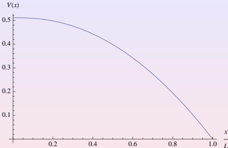
Figure: Fundamental flapping shear mode shape of a rotating clamped-free beam with zero hub offset for  $\Omega = 25\sqrt{\frac{EI}{mL^4}}$
