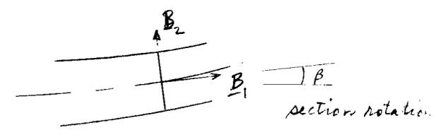
$\underline{B}_1$  is normal to the cross section plane ( $\underline{B}_2$  lies in that plane)
