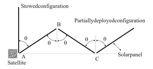
Figure 1: Satellite in stowed and deployed configurations
