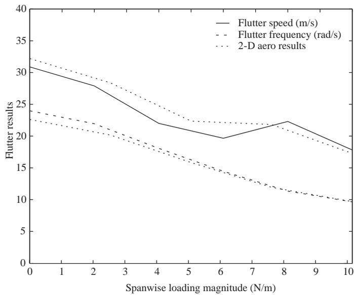
Fig. 5. The effect of geometrical nonlinearities on flutter.
