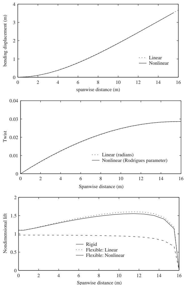
Fig. 2. Comparison between linear and nonlinear equilibrium for the wing at a speed of 25 m/s and angle of attack of  $2^\circ$ .
