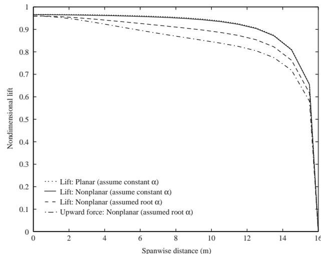
Fig. 1. The effect of geometrical nonlinearities on the lift generated by a curved rigid wing.
