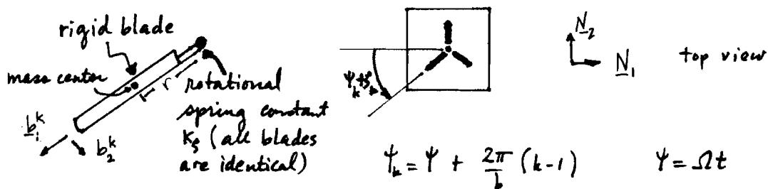
A simple system that will exhibit the "ground resonance" instability is shown above. Let each blade have one degree of freedom  $\xi_k$ . The rotating unit vectors are related to the fixed ones
