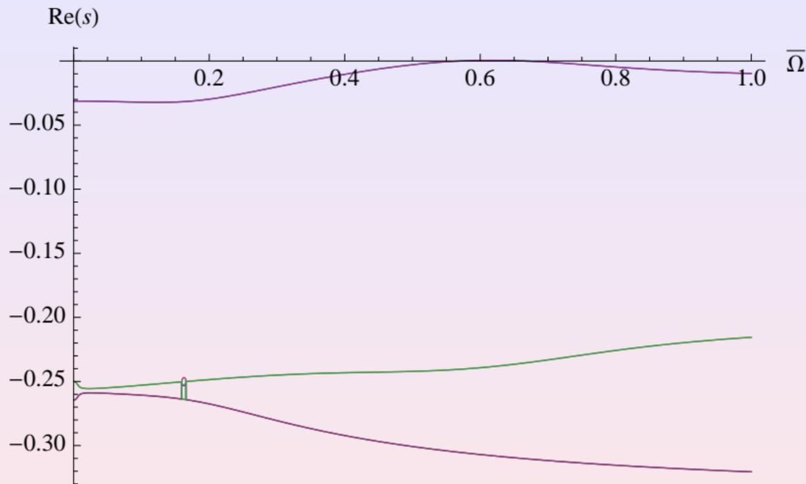
Figure: Modal damping for  $\mu = 0.3$ ,  $\omega_\zeta = 0.3$ ,  $\omega_X = 0.4$ ,  $c_X = 0.025$ ,  $c_\zeta = 0.5$
