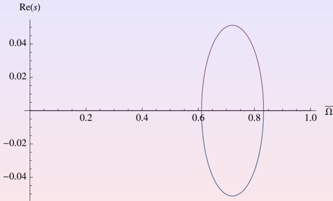
Figure: Modal frequency for  $\mu = 0.3$ ,  $\omega_{\zeta} = 0.3$ ,  $\omega_X = 0.4$
