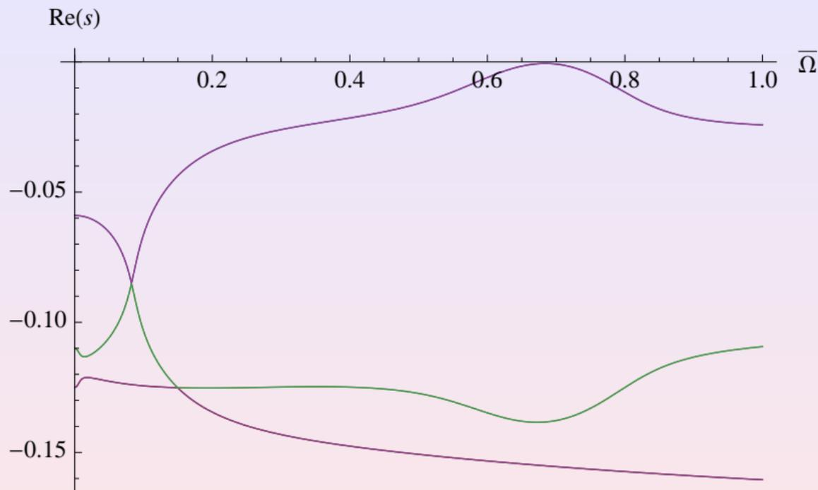
Figure: Modal damping for  $\mu = 0.3$ ,  $\omega_\zeta = 0.3$ ,  $\omega_X = 0.4$ ,  $c_X = 0.05$ ,  $c_\zeta = 0.25$
