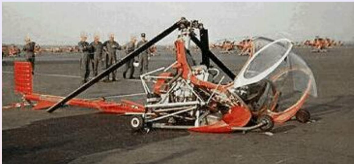
Figure: Catastrophic destruction from ground resonance
