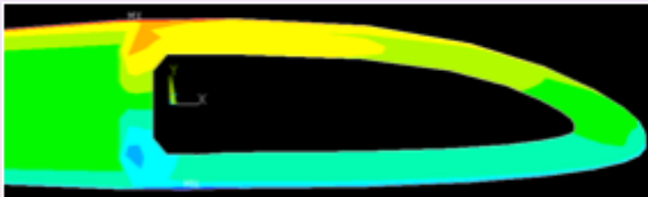
Figure: Sample stress output from cross-sectional analysis VABS
